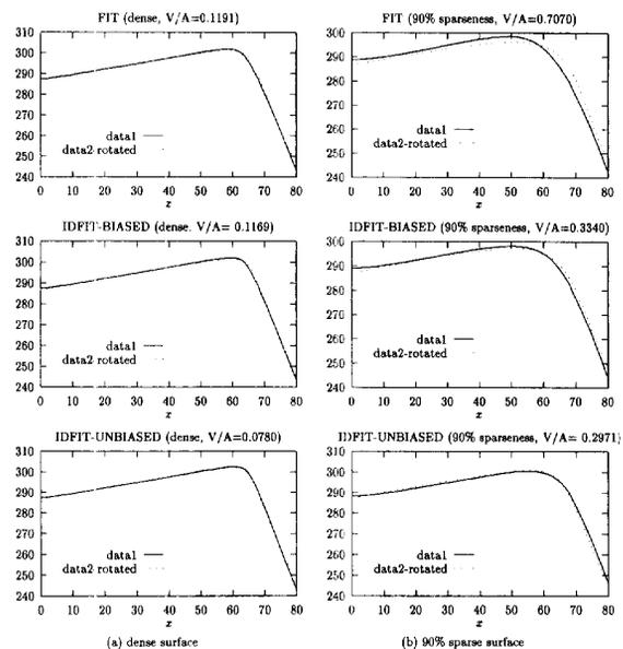
Fig. 5. Invariance performance of FIT, IDFIT-BIASED, and IDFIT-UNBIASED,  $\lambda = 3.0$ . In order to show the invariance performance of three methods, dense and sparse DATA1 and DATA2 that are noisy are reconstructed and the reconstructed result for DATA2 is rotated back into correspondence with DATA1. Comparison of a section of the reconstruction results is displayed. The vertical axis represents  $z$  value.
