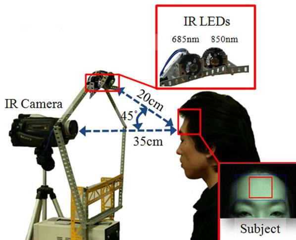
Fig. 11. (Color online) Sketch of the experimental setup.
